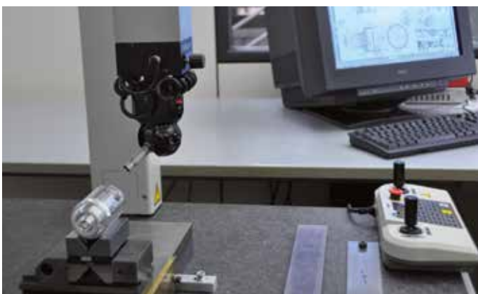
Inspection of a hydraulic pump core by 3D device
