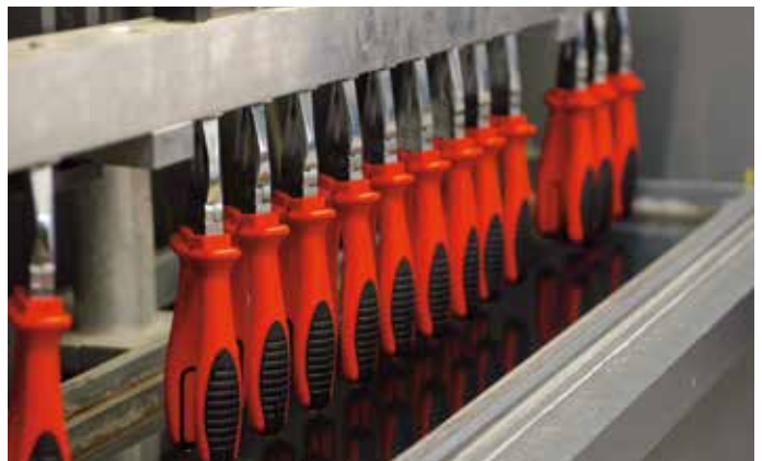
10.000V voltage test
